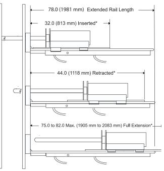
\*Variable length, dependent on placement of camera on Retract Mechanism
