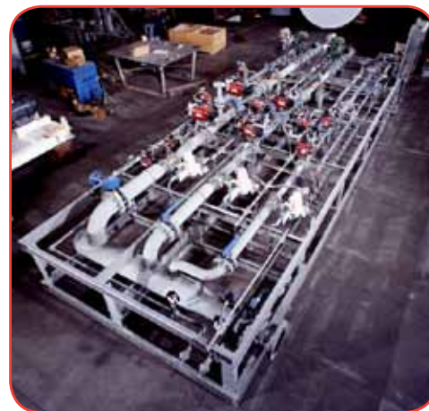
Fuel Piping / Control Skid
